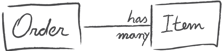
Figure 2.38 First draft of a conceptual data model. This and the next two diagrams are fragments of an online order-processing system at different stages.
